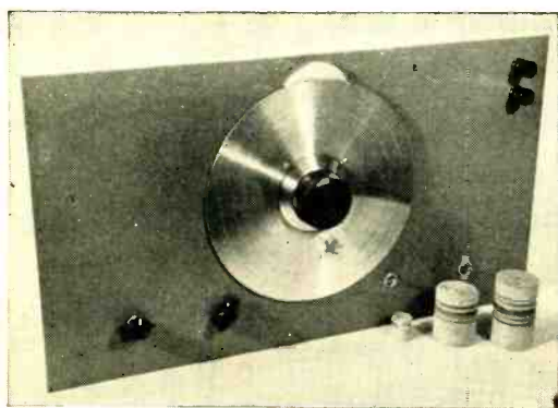
Front view of the unit showing the large dial (un-engraved). Three of the unwound coil forms are also shown in front of the panel.
